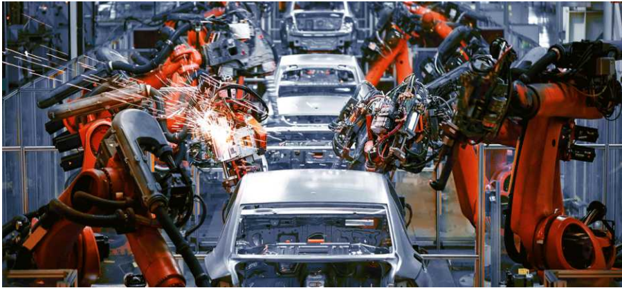
Automation already exists in a major way in manufacturing. Here, robotic arms manufacture car bodies in a factory in Ontario
