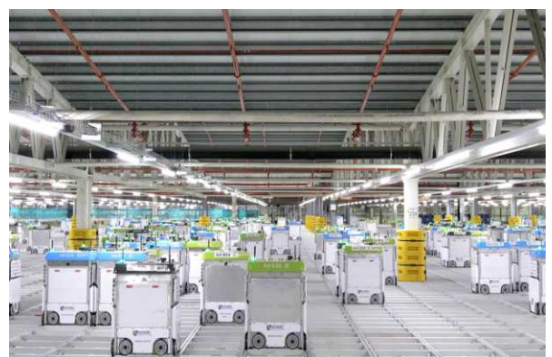
This Ocado warehouse is entirely run by machines. Customer orders are recieved and the robots move around on grids to pick up groceries and items. It then packages the items and leaves them for human drivers to deliver.
